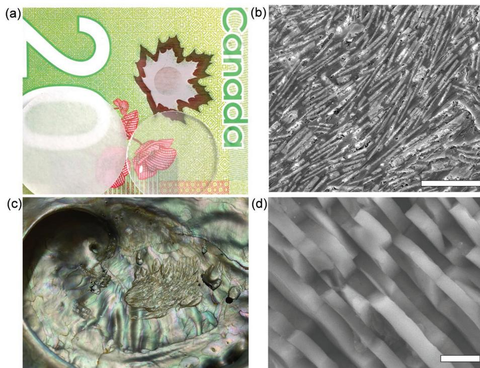
**Figure 12.** Nacreous composites for tough transparent glass. a) PMMA–glass composite with PMMA index matched to glass (top, transparent) or neat state (bottom, translucent). b) SEM microstructure of glass flakes connected in PMMA continuum. c) Natural nacre surface. d) SEM microstructure of well-ordered brick and mortar natural nacre structure. The scale bars in (b) and (d) are 20  $\mu\text{m}$  and 3  $\mu\text{m}$ , respectively.
