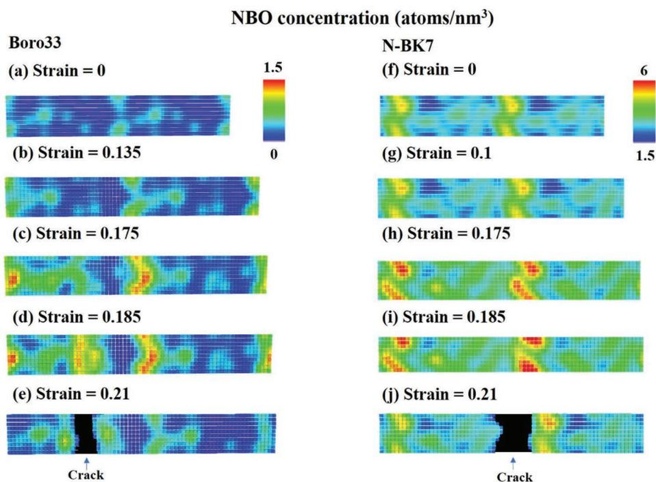
**Figure 8.** MD-simulated evolution of NBO distributions (atoms nm<sup>-3</sup>) during uniaxial tension tests for Boro33 and N-BK7 borosilicate glasses. The samples fractured at the strain of 0.21. Reproduced with permission.<sup>[134]</sup> Copyright 2020, John Wiley & Sons.
