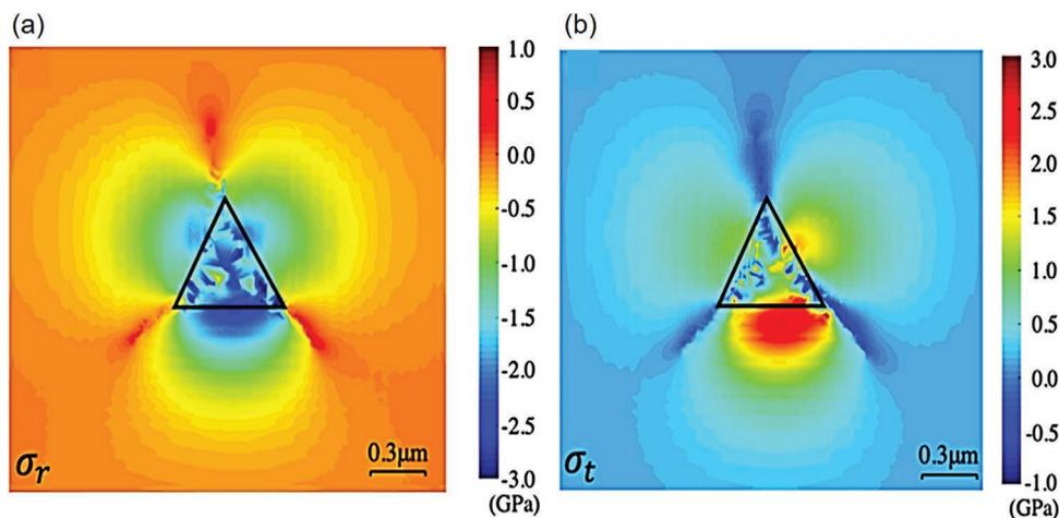
**Figure 9.** Peridynamics calculated a) radial and b) tangential stress distribution in the plane along which the indenter tip enters in contact with the soda-lime silicate glass. The resulting stress is localized at the vicinity of the indenter (black triangle indicates the extent of the projected contact area with the indenter). Reproduced with permission.<sup>[152]</sup> Copyright 2021, John Wiley & Sons.
