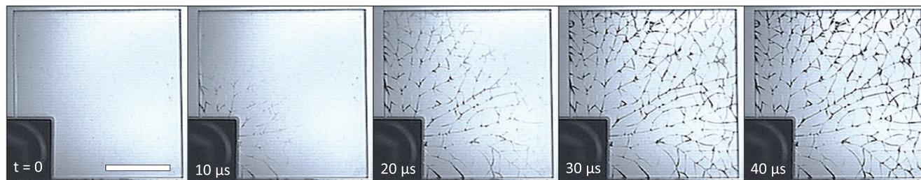
**Figure 6.** Video frame sequence of a fracture event observed in a thermally strengthened borosilicate glass sheet of 3.3 mm thickness. Collected in diffuse transmission mode at a rate of  $10^5 \text{ fps}$ . The scale bar is 20 mm.
