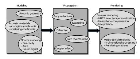
Fig. 2.1: A general pipeline for sound simulation in Virtual Reality (figure based on [51]).
