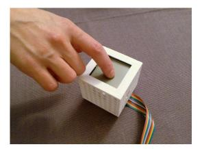
**Fig. 12.4** The interface used in the experiment for recording finger-pressing force and providing vibrotactile feedback.
