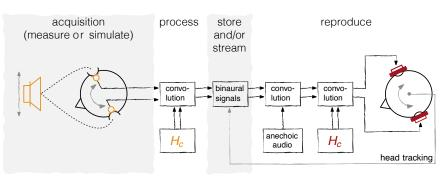
Fig. 5.11: Example of a headphone based pipeline for binaural synthesis. Dashed lines indicate acoustic signals; black lines indicate digital signals; gray lines indicate movements in 6DoF.  $H_c$  denote compensation filters for the recording (yellow) and reproduction equipment (red, CC-BY, Fabian Brinkmann).
