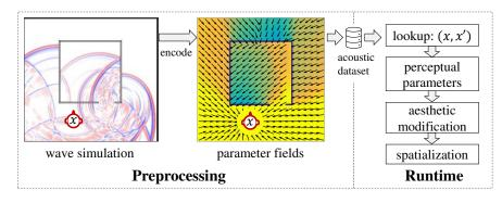
Fig. 3.4: High-level architecture of Project Acoustics' wave-based parametric auralization.
