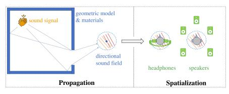
Fig. 3.1: Modular architecture of real-time auralization systems. The propagation of sound emitted from each source is simulated within the 3D environment to compute a directional sound field immersing the listener. This field is given to the spatializer component that computes appropriate transducer signals for headphone or speaker playback.
