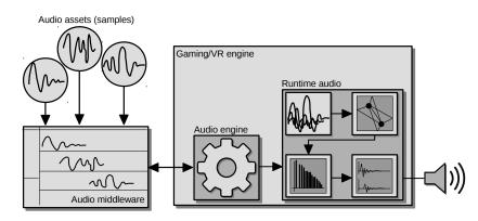
Fig. 2.5: Event-driven logics for VR sound design using samples and audio middleware software.
