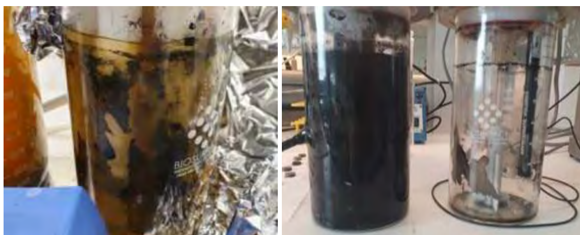
Figure 11: (A) Bioreactor which was continuously treated with the halophyte extracts in growth medium for after 1 week (B) Comparison between bioreactors after experiment concluded and bioreactors were emptied. From left, bioreactor treated with halophyte extracts for 4 hours twice per week, and a bioreactor with halophyte extract added to growth medium. The first exhibit no discernable difference from before extracts were added.
