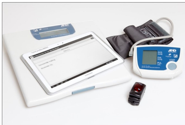
Fig. 1 The telehealth system, Telekit, consists of a tablet, a fingertip pulse oximeter, a blood pressure monitor, and a scale
