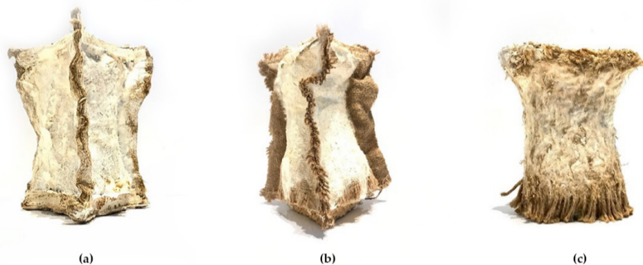
Figure 6. Results of grown on different skin materials: (a) hemp sheets, (b) jute sheets, (c) knitted hemp rope.
