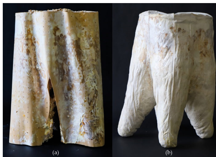
Figure 1. Mycelium-based prototypes: (a) using a timber veneer mold, and (b) using cotton fabric mold, by F. Milano, K. Antorveza, L. Kiesewetter, G. Lochnicki, Materials Matter Lab IV, 2020.
