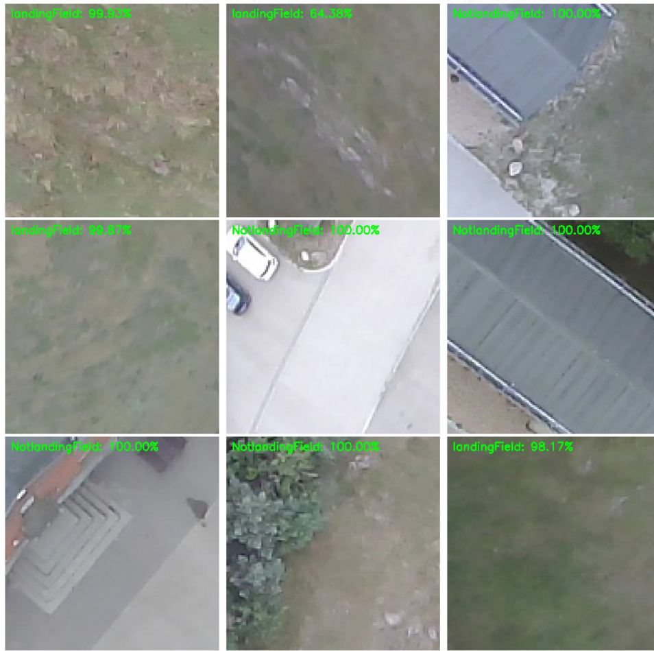
Figure 15. Results of the percentage of confidence in the classification from the image classifier after the model trained with the dropout layer and updated images from the new test flights.
