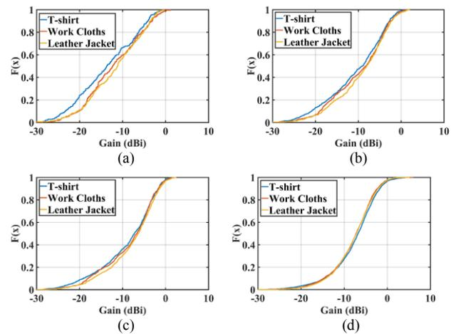
Fig. 14. The comparison of CDFs of human's blockage patterns for different types of clothes within the window size of (a) 40°, (b) 80°, (c) 140°, and (d) 360°.
