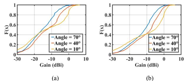
Fig. 18. The comparison of CDFs of phantom blockage pattern for different relative angles to the horizon for window size of (a) 80°, (b) 140°.
