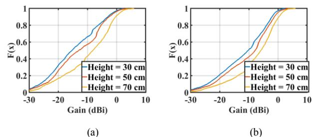
Fig. 17. The comparison of CDFs of phantom blockage pattern for different heights for window size of (a) 80°, (b) 140°.
