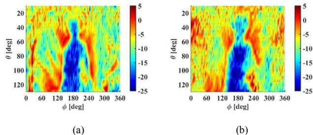
Fig. 4. The blockage pattern of (a) phantom with torso height of 81 cm, and (b) human subject with torso height of 84 cm.
