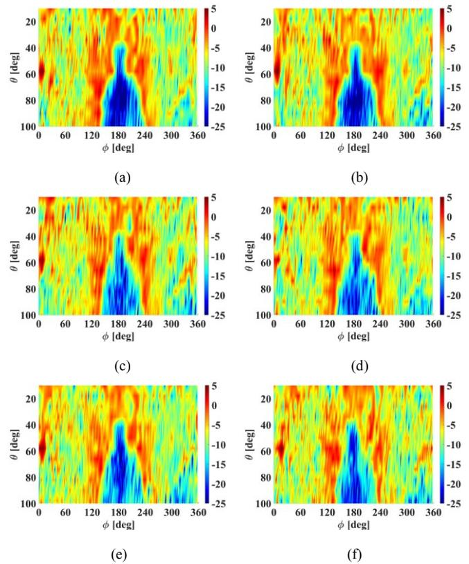
Fig. 13. The blockage patterns of the phantom (a) without clothes, and phantom with (b) T-shirt, (c) raincoat, (d) work clothes, (e) leather jacket, and (f) winter jacket.
