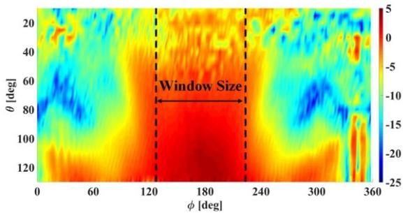
Fig. 3. The antenna free space radiation pattern.
