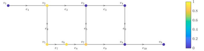
Fig. 5. The leakage localization indicators for each node for the laboratory test.
