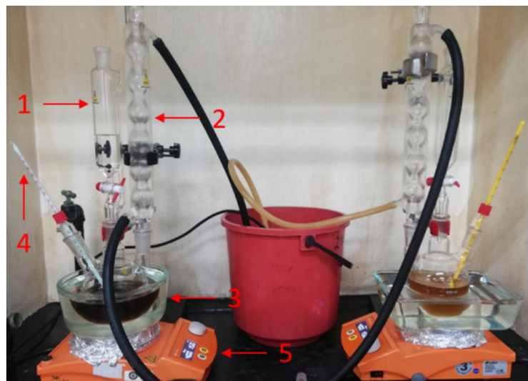
Figure 2. Experimental system reported in [11], including (1) a methanol/KOH mixture container, (2) reflux condenser, (3) heating bath, (4) temperature controller, and (5) magnetic stirrer
