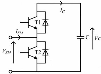
Fig. 2. Basic building block of MMC: Power sub-module
