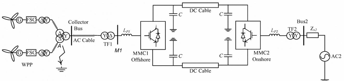
Fig. 1 MMC based HVDC system for WPP connection
