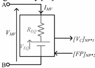
Fig. 6 Thévenin equivalent of a multi-valve of MMC
