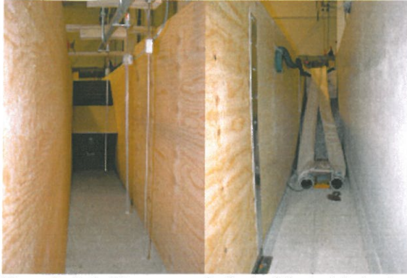
Figure 5: Left: Wave gauges in front of the tested structure (note the limited draught of the ramp). Right: Pipes from the pumps emptying the tanks. Thus, the overtopping water is returned to the flume between guiding wall and sidewall of the flume.
