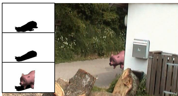
Figure 3: A virtual pig is augmented into a scene, to create the shadow effect, the shadow of the surroundings are subtracted from the pig's and blended into the image. Furthermore the surroundings cast shadow on the pig.
