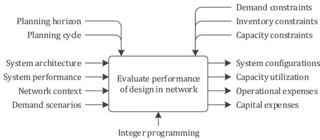
Fig. 1. IDEFO representation of proposed optimization model.
