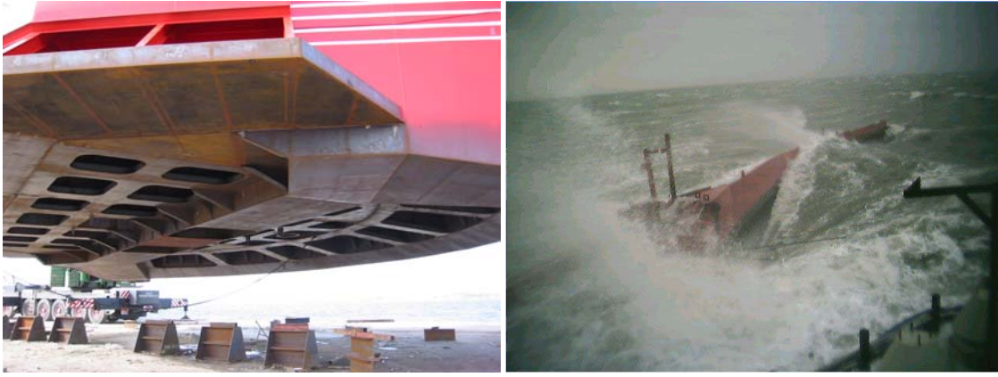
Figure 4. Left: WD prototype at launch in March 2003. The open air-chambers are used to control the floating level. Right: WD prototype in heavy wave conditions.
