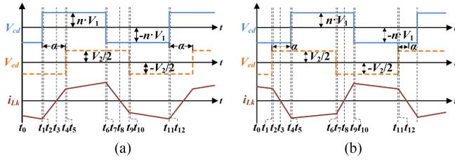
**FIGURE 5.** Typical waveforms when  $2 \cdot n \cdot V_1 / V_2 > 1$ . (a) Forward mode, i.e.,  $0 < \alpha < T_s/4$ . (b) Backward mode, i.e.,  $-T_s/4 < \alpha < 0$ .
