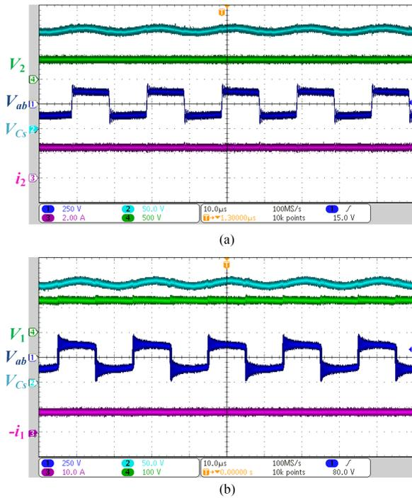
**FIGURE 10.** Steady state waveforms of the proposed converter under rated work conditions. (a) Forward mode ( $P_2 = 1$  kW). (b) Backward mode ( $P_1 = 1$  kW).
