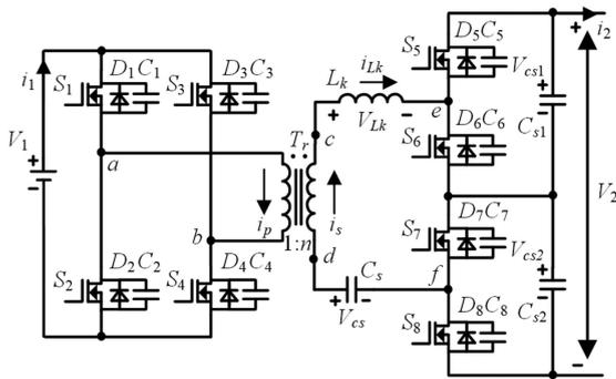
**FIGURE 2. Circuit structure of proposed converter.**
