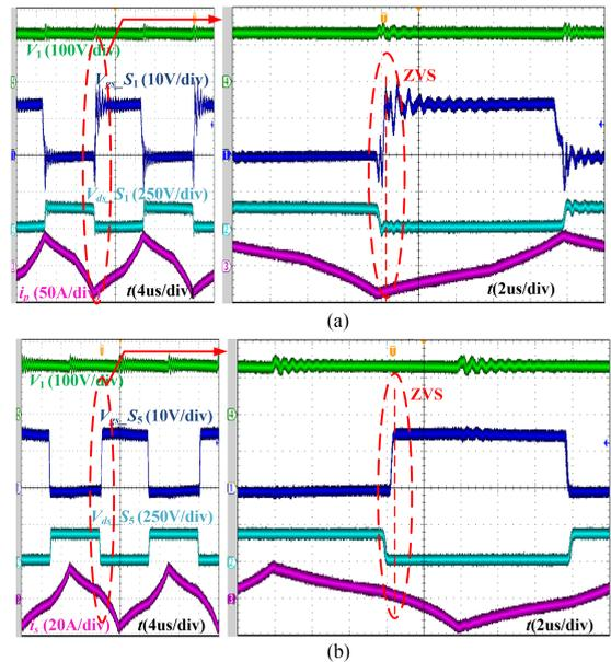
**FIGURE 13.** Driving signal and drain-source voltage of main switches when  $V_1 = 128$  V,  $V_2 = 400$  V,  $P_1 = 1$  kW in backward mode. (a)  $S_1$ . (b)  $S_5$ .
