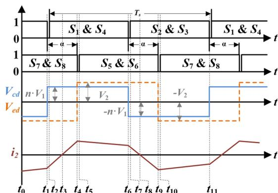
**FIGURE 17. Typical operating waveforms of traditional NPC converter in forward mode.**
