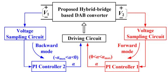
FIGURE 9. Control block diagram for proposed converter.
