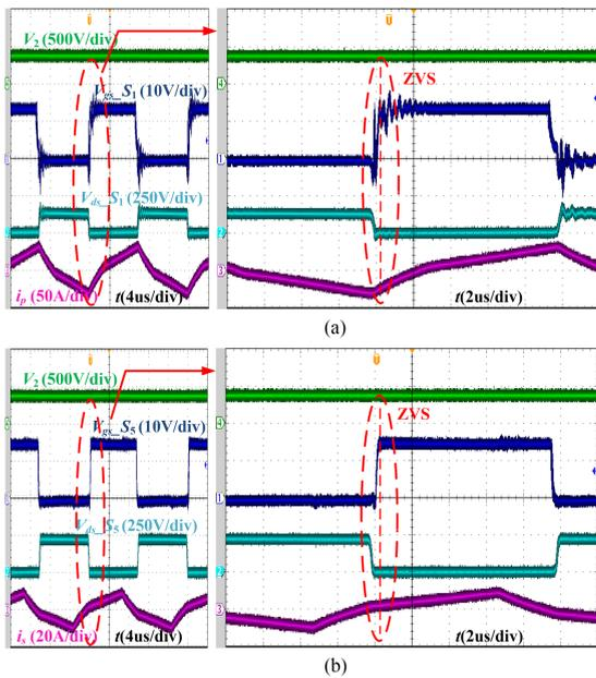
**FIGURE 11.** Driving signal and drain-source voltage of main switches when  $V_2 = 400$  V,  $R_2 = 160\Omega$ ,  $P_2 = 1$  kW in forward mode. (a)  $S_1$ . (b)  $S_5$ .
