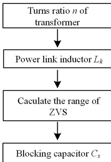
**FIGURE 7.** The design process of key parameters.
