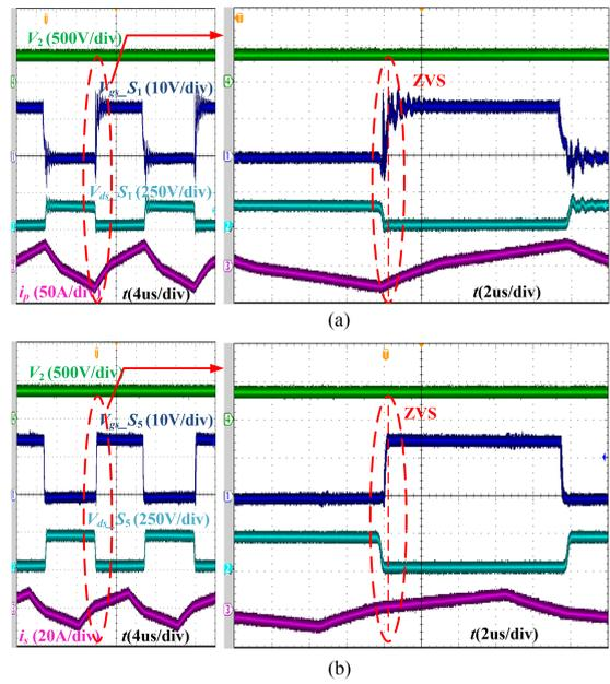
**FIGURE 12.** Driving signal and drain-source voltage of main switches when  $V_2 = 360$  V,  $R_2 = 160\Omega$ ,  $P_2 = 810$  W in forward mode (a)  $S_1$ . (b)  $S_5$ .
