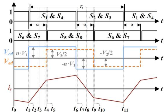
**FIGURE 3. Typical operating waveforms when  $2 \cdot n \cdot V_1 / V_2 > 1$  in forward mode.**
