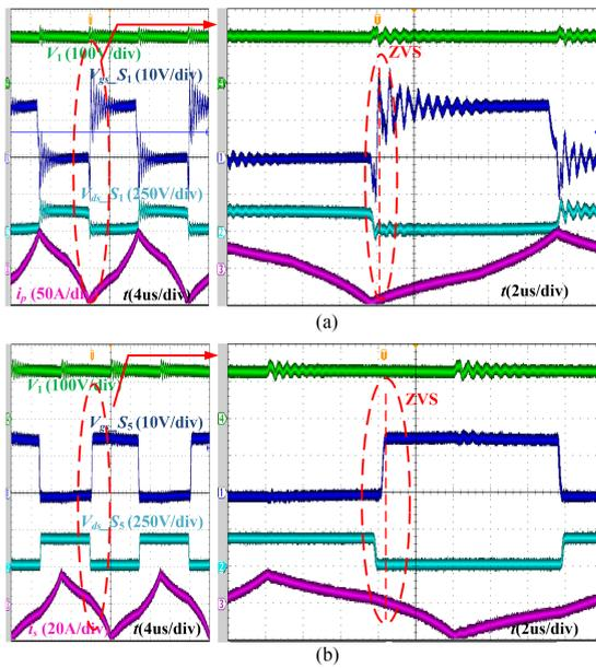
FIGURE 14. Driving signal and drain-source voltage of main switches when  $V_1 = 128\text{ V}$ ,  $V_2 = 360\text{ V}$ ,  $P_1 = 1\text{ kW}$  in backward mode. (a)  $S_1$ . (b)  $S_5$ .
