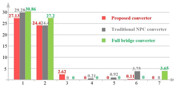
FIGURE 15. Comparison results about loss breakdown when  $V_1 = 128\text{ V}$  and  $V_2 = 400\text{ V}$ . Note: 1. Total loss of main devices in secondary-side 2. Power switches' loss; 3. Blocking capacitor's loss; 4. Clamping capacitor's loss; 5. Clamping diodes' loss; 6. Dividing capacitors' loss; 7. Output capacitor's loss.
