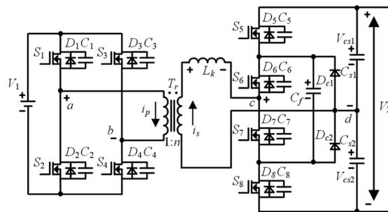
FIGURE 1. Conventional hybrid-bridge based DAB DC/DC converter with a diode-clamped TL structure.
