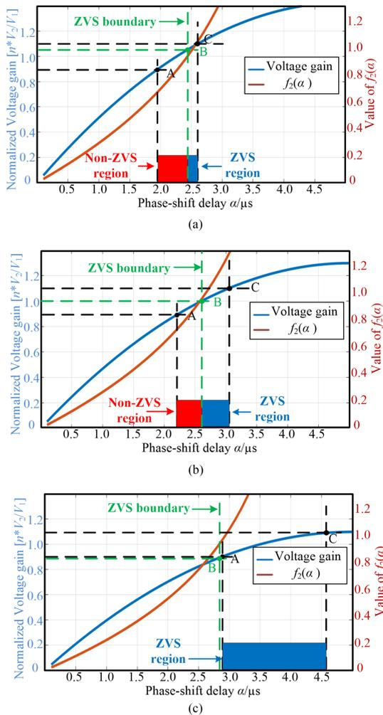
**FIGURE 6.** ZVS boundary of  $S_5$ ,  $S_6$ ,  $S_7$ , and  $S_8$  with different  $L_k$  under forward mode. (a)  $L_k = 140 \mu\text{H}$ . (b)  $L_k = 153 \mu\text{H}$ . (c)  $L_k = 179 \mu\text{H}$ .
