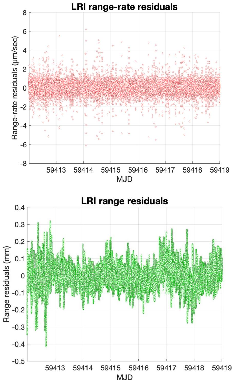
**Fig. 4.** GRACE-FO intersatellite observations residuals per epoch to the estimated orbits of a weekly period. The intersatellite range and range-rate data are obtained from the Laser Ranging Interferometry (LRI) instrument. RMS values are 0.43  $\mu\text{m/s}$  and 0.08 mm for range-rate and range residuals respectively. Units are  $\mu\text{m/s}$  and mm for range-rate and range residuals respectively.
