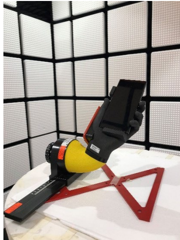
Figure 5: Data mode with phone placed in the left-hand phantom (LH).
