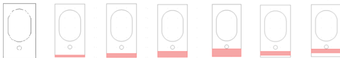
Fig. 5. COMSOL models: Model without PCM and with highlighted various location and thickness of layer with combined concrete and PCM.
