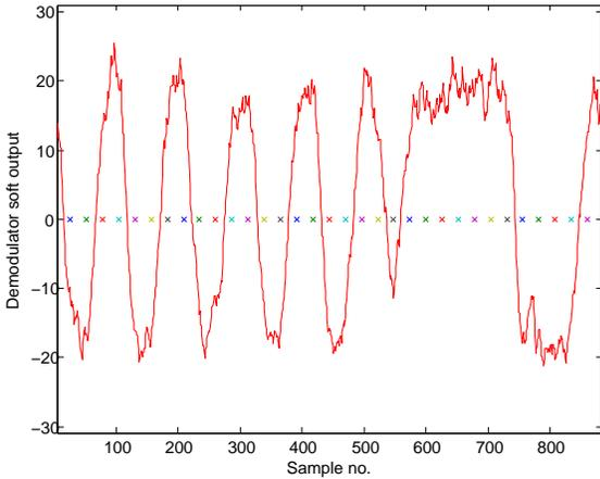
Figure V: Start of AIS package, demodulated by AIS2.
