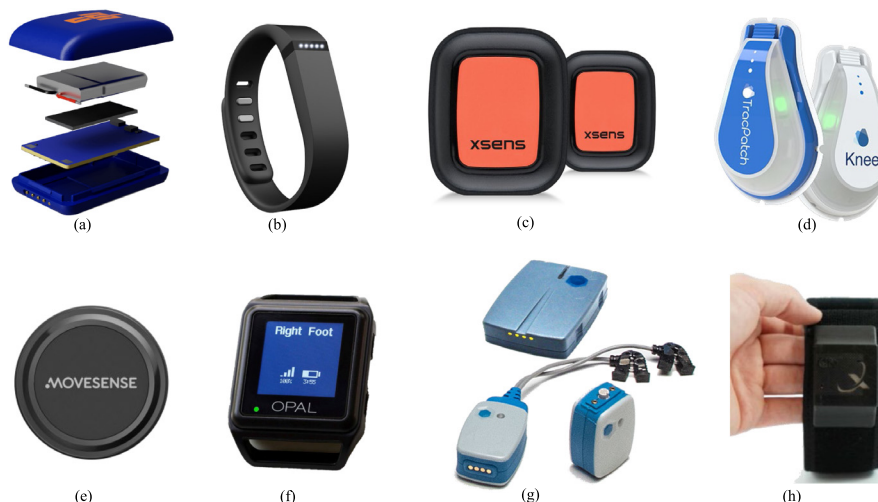
Fig. 4. Typical commercial wearable devices for activity monitoring and tracking. (a) Vicon; (b) Fitbit Flex; (c) XSens; (d) TracPatch; (e) Movesense; (f) APDM; (g) Noraxon; (h) BioX Bands.
