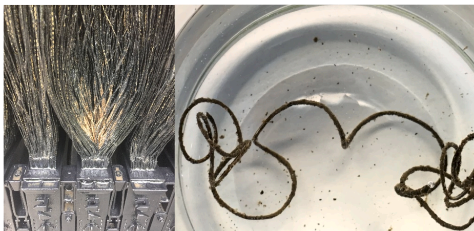
Fig. 6. Membrane samples with a seemingly black coating from R1 and R2 sampled during P1.
