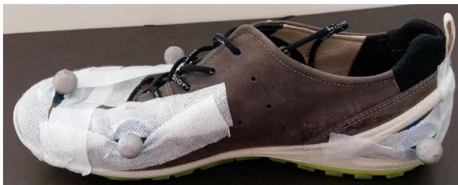
Figure 7: Five retroreflective markers were affixed to the right shoe: toe, 1 st and 5 th metatarsal, medial and lateral calcaneus (study 4).
