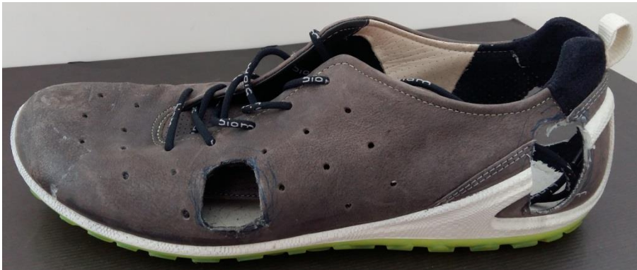
Figure 3: Left shoe with large enough holes for 5 th metatarsal and calcaneus displacement monitoring (study 3 and study 4).
