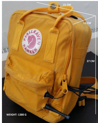
Figure 2: Backpack including minicomputer (UMPC-ViliV) and Stand-Alone Wireless Sync-Trigger system (Noraxon), 1380 g total weight with dimensions indicated in the picture.
