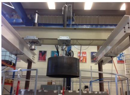
**Figure C.8** The installation of bucket  $d/D=0.5$ .
