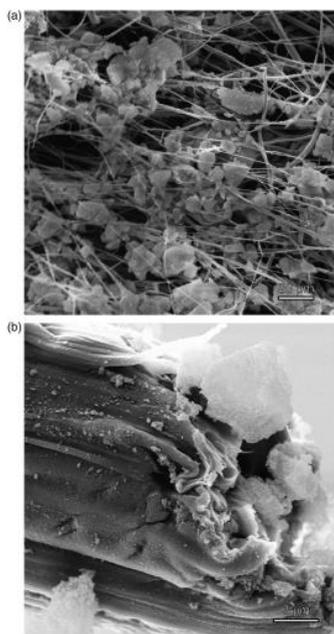
**Figure 5.** Blow spun fibers with aerogel pneumatically transported into the spinning nozzle. (a) An overview image showing the aerogel distributed in the fiber network and (b) a magnified image of a fiber in cross-section, which shows aerogel is located both inside and outside of the fiber.
