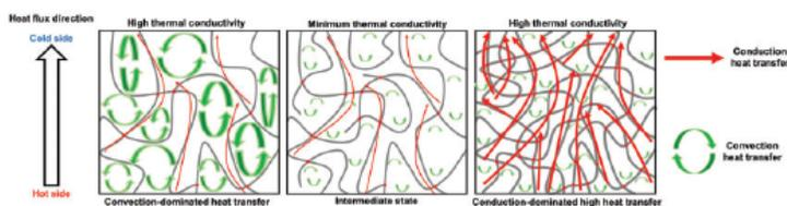
**Figure 1.** Illustration of two hypothesized states of porosity and pore structure during compression of fibre material. Red arrows represent conduction, green convection. Less compacted and convection dominated pore network (left); higher compaction and conduction-dominated pore network (right). In the middle, an intermediate state where the sum of the two has a minimum thermal conductivity.
