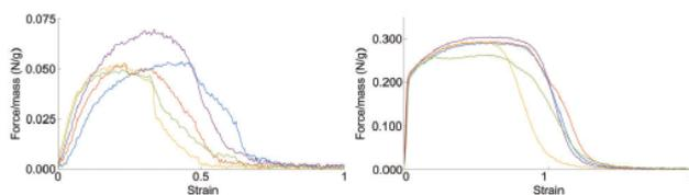
**Figure 7.** Force per mass as a function of strain: Left) PET-aerogel blow spun fibers and Right) PET reference fibers. It is seen that the composite fibers have a force per mass ratio for failure four to five times lower than the reference fibers.
