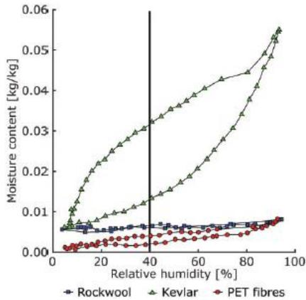
**Figure 4.** Water vapour adsorption and desorption isotherms for the three fibre materials. The vertical solid line at 40% relative humidity marks the laboratory ambient conditions while running of the thermal tests. Note the connected data points to show adsorption and desorption, and that these isotherms are similar for Rockwool.
