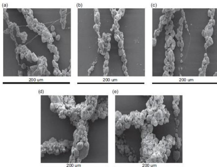
**Figure 2.** SEM images of fibres spun from Solution 5 with polymer/particle weight ratio 1:8. They are spun at different flowrates: (a) 0.25 mL/h, (b) 0.50 mL/h, (c) 1.00 mL/h, (d) 1.50 mL/h and (e) 2 mL/h. It is seen that higher flowrates in general promoted thicker fibres. All images are 200  $\mu\text{m} \times 200 \mu\text{m}$ .
