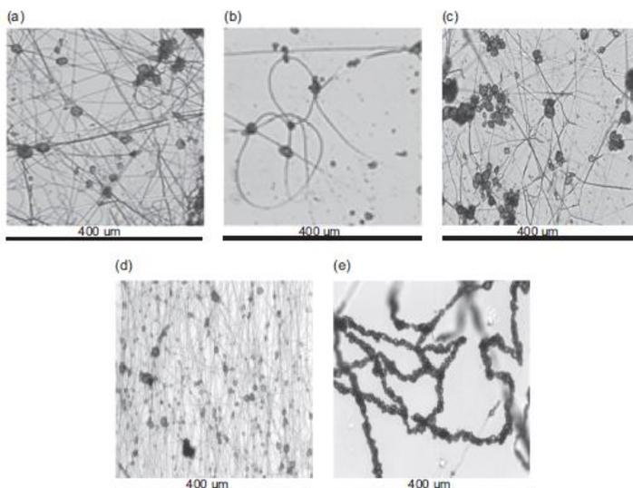
**Figure 1.** Optical microscopy of fibres spun from polymer/silica aerogel particle solutions with weight ratios (a) 1:1, (b) 1:2, (c) 1:4, (d) 1:6 and (e) 1:8. It is seen that the amount of particles increases until the silica aerogel particles packs closely in the fibre.
