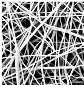
Figure 3. Reference fibers electrospun from PET solution.
