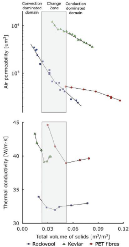
**Figure 6.** Thermal conductivity and air permeability as a function of volume content of solids for fibre materials. The shaded area is the change zone. The change point for PET fibres is marked at the first data point, as this measurement was in overflow. Note: Logarithmic y-axis for air permeability, and tendency lines for air permeability are piecewise exponential.
