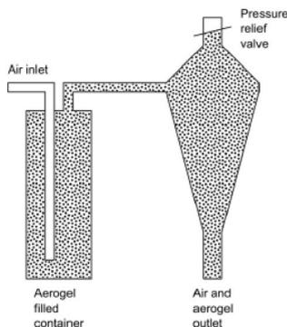
**Figure 2.** The aerogel inlet system. Nitrogen travels through a rinsing flask filled with aerogel. It is conveyed into a funnel, ending in a piece of tubing, keeping the aerogel nitrogenborne into the spinning needle.
