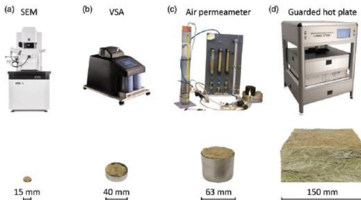
**Figure 2.** Instruments used for characterization of the material properties with a typical size of test samples for fibre materials. For illustration purposes, Rockwool<sup>®</sup> is used.
