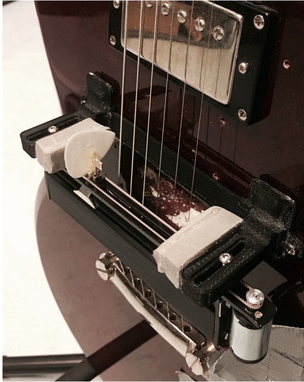
Fig. 4.11: Foam stopper were added to each end of the fader to reduce noise and latency.
