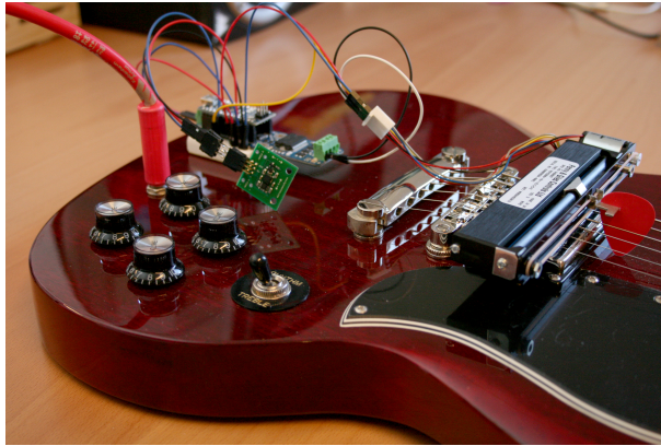
Fig. 4.3: The first proof of concept of the Actuated Guitar testing out different types of input, in this case an accelerometer.
