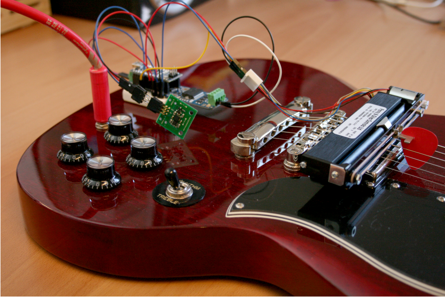
Fig. 2.4: An Arduino capturing human gestures with an accelerometer enabling people to strum the guitar who otherwise would not be able to.
