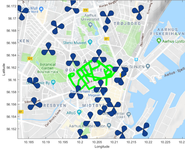
Fig. C.1: Measurement route (in green) in Aarhus (Denmark), including LTE network sites location provided by a local operator.
