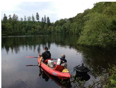
Picture 3-4 Field sampling for phytoplankton and measurements of water quality parameters: conductivity, pH, dissolved oxygen, temperature.
