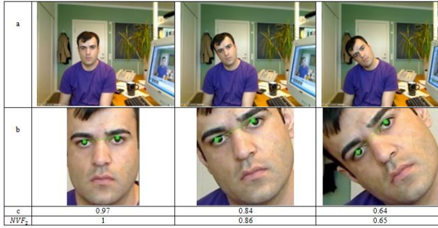
Figure 4-5: Changes in the head tilt of a given sequence: a) input sequence, b) detected center of mass of the eyes and c) T_i .
