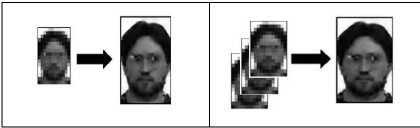
Figure 6-4: Recognition-based (left) vs. Reconstruction-based (right) super-resolution algorithms
