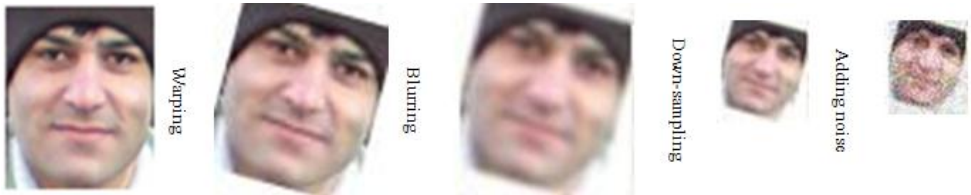
Figure 7-1: The imaging model. The desired high-resolution image is at the extreme left and the observed low-resolution image is at the extreme right.
