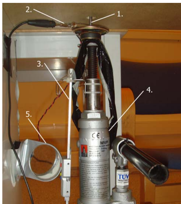
Fig. 3 The setup. 1 The stainless steel bolt attached to the pc speaker, 2 a cord connecting an ohm meter to the bolt, 3 a digital ruler, 4 the jack, 5 a mirror used for reading the digital ruler while operating the setup
