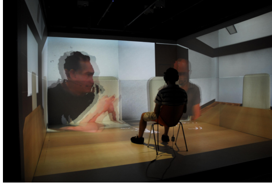
Fig. 1: The setup at the visitor's side in the CAVE. The image looks blurry due to the stereoscopic image. The visitor is wearing 3D glasses, headphones and a headtracker.
