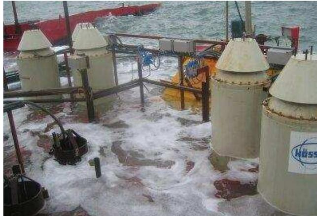
Fig. 11: Turbines in the reservoir of the prototype: The yellow structure in the background is the siphon turbine, the grey towers are five of the six cylinder gate turbines, and the small devices in unpainted steel are two of the dummy turbines.
