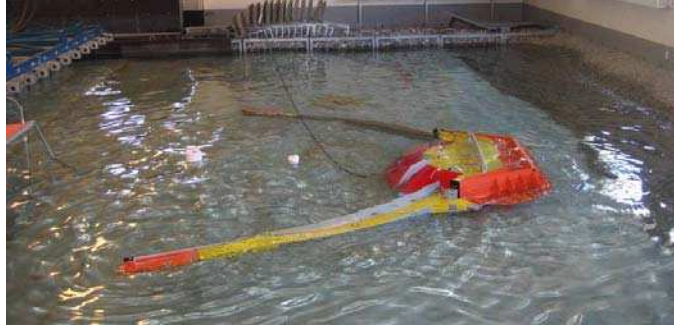
Fig. 4: Testing of 1:50 scale Wave Dragon in Aalborg University wave basin.
