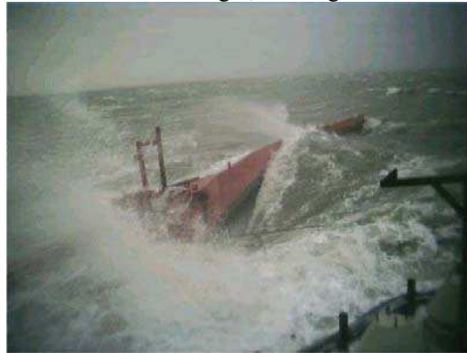
Fig. 3: View from web camera mounted to control container of large wave surging down reflector wing of Wave Dragon.
