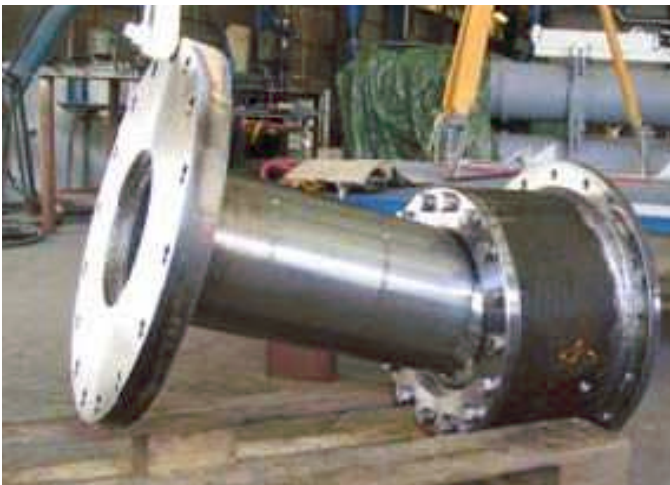
Figure 10: Manufactured joint and fitting on main platform.
