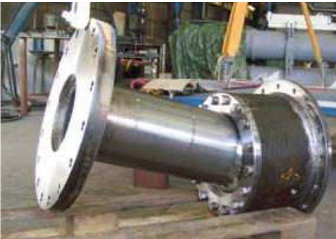
Figure 10: Manufactured joint and fitting on main platform.
