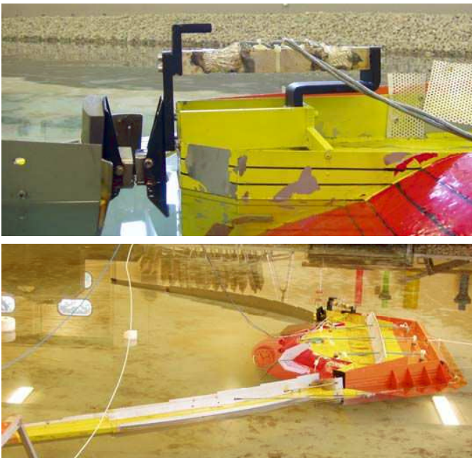
Figure 5: Test setup with 1:51.8 scale model and force transducer measuring shear force at joint
