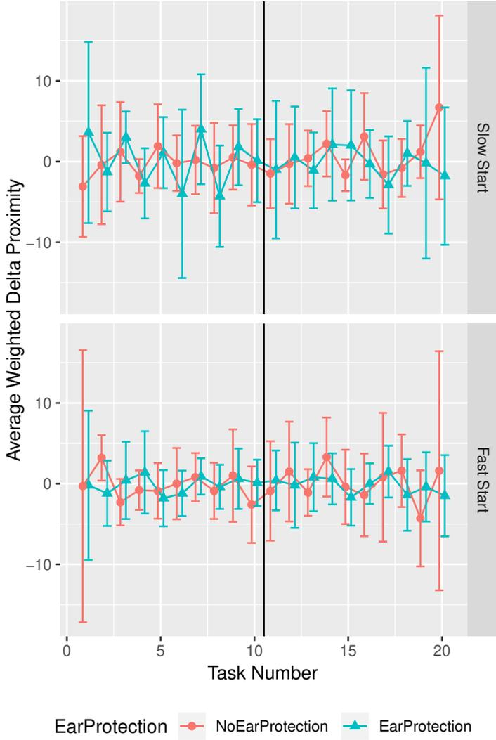
**Fig. E.6:** Average participant motion for the first second of robot movement weighted by movement direction along with confidence interval. The vertical lines mark the midway point of the test where the robot speed ratio changes.
