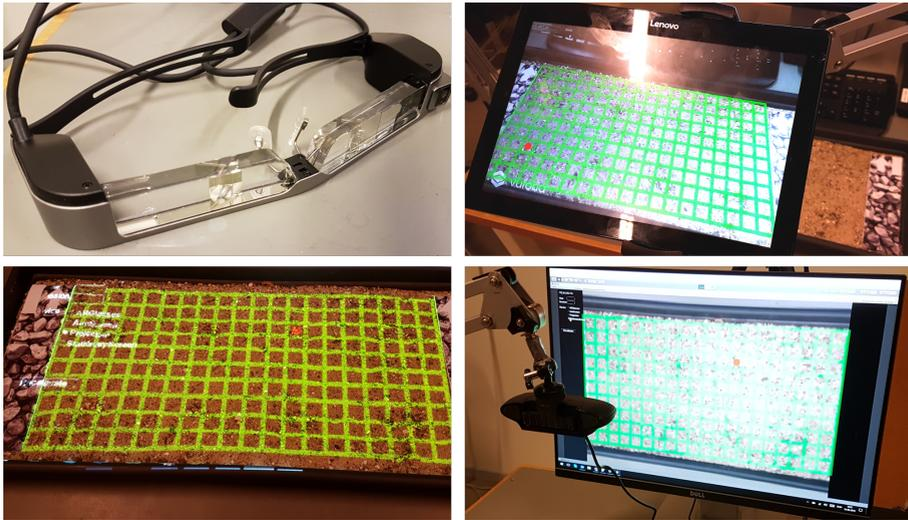
**Fig. 3.3:** The four AR display types evaluated in the experiment. Top-left: Epson Moverio Bt-300 see-through HMD with camera. Top-right: Android tablet with back-camera feed on adjustable arm. Bottom-right: Projected overlay on the surface of the sand. Bottom-right: Top-down camera feed with overlay on monitor. © 2019 Springer, Cham [5]
