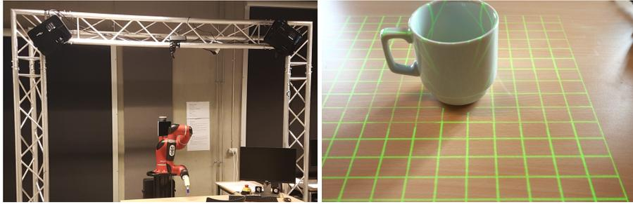
**Fig. 3.1:** Left: Full HRC cell setup with Sawyer robot, projectors and infrared camera. © 2020 IEEE [6]. Right: A coffee cup sitting under the dual-AR projection, preventing the cup from occluding either side of the AR overlay.
