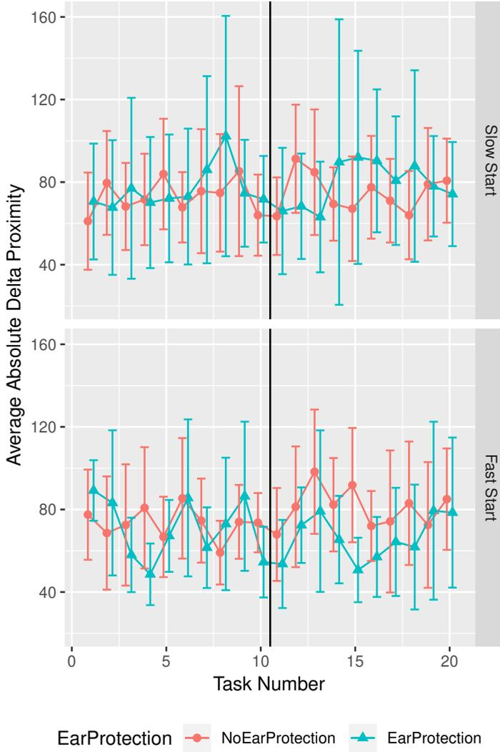
**Fig. E.7:** Average absolute participant motion for the first second of robot movement along with confidence interval. The vertical lines mark the midway point of the test where the robot speed ratio changes.
