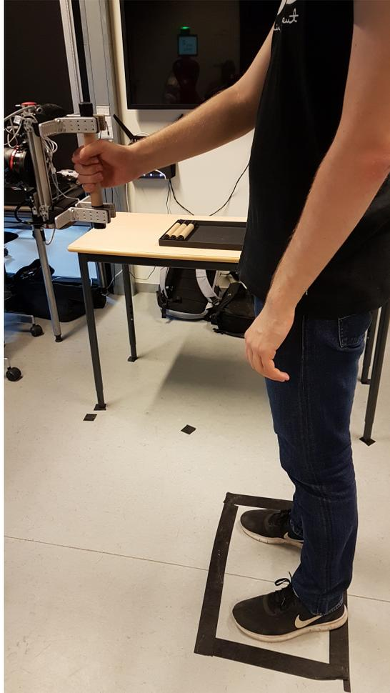
**Fig. D.1:** A test participant standing with the marked zone on the floor, grabbing the baton from the robot in the condition with no table in-between.
