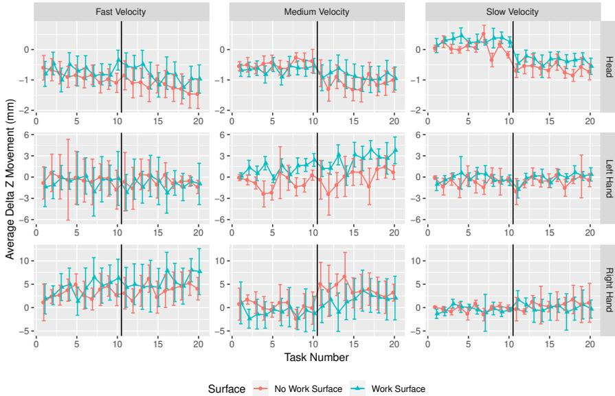
**Fig. D.3:** Average delta motion towards and away from the robot of the participants' head and hands for the first two seconds after the robot starts moving, negative being away from the robot. Includes confidence intervals.
