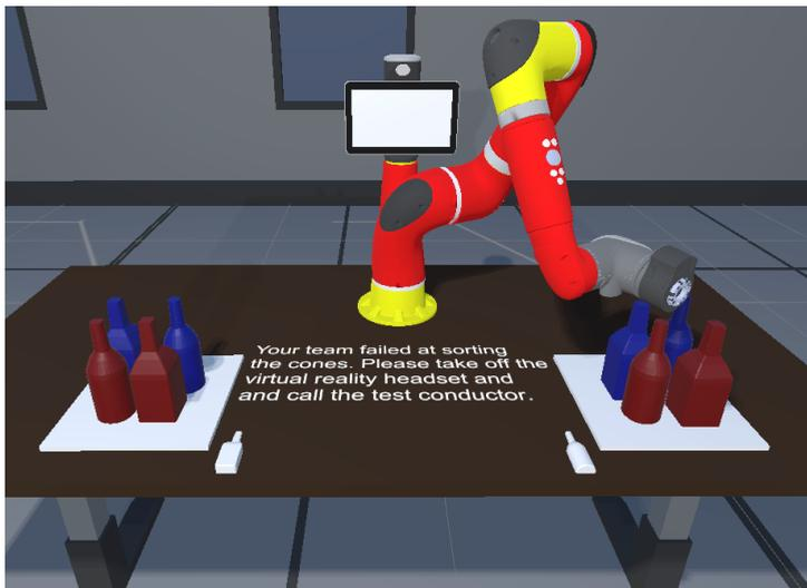
**Fig. 3.2:** The virtual environment and virtual robot used to test mistake explanations for trust repair. The bottles had to be sorted with round bottles on the right and square bottles on the left. The space between the two bottle areas allows for displaying text for communicating with the participant [7].
