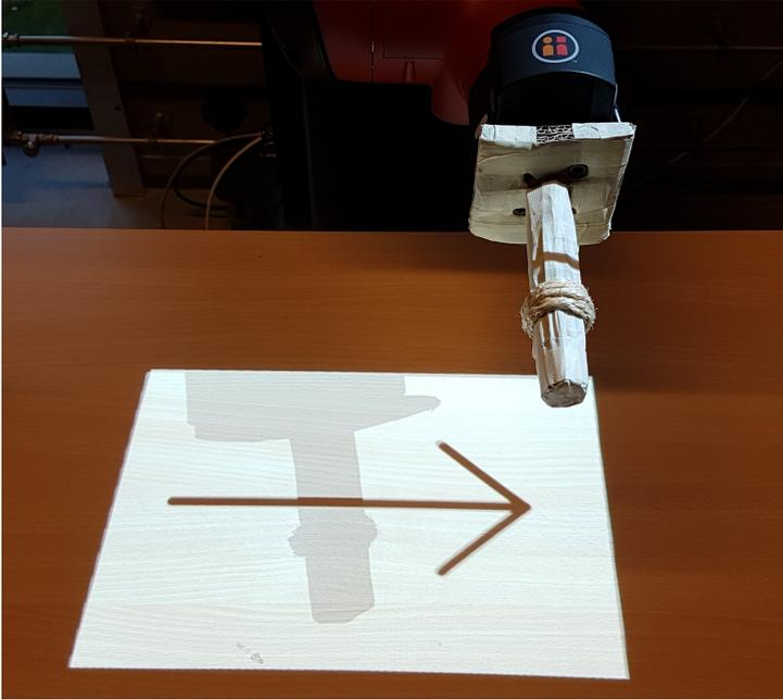
**Fig. F4:** The rod mounted to the robot for picking up and moving the cones. The augmented reality overlay is made with two overlapping projections from the projectors mounted at either side of the aluminum rig and pointed diagonally down, as shown in Figure F.1, making the projection harder to occlude.
