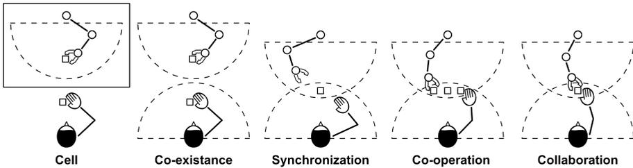
Fig. 1.3: The five levels of engagement in HRC, illustrating the overlapping work spaces of the operator and robot [6].
