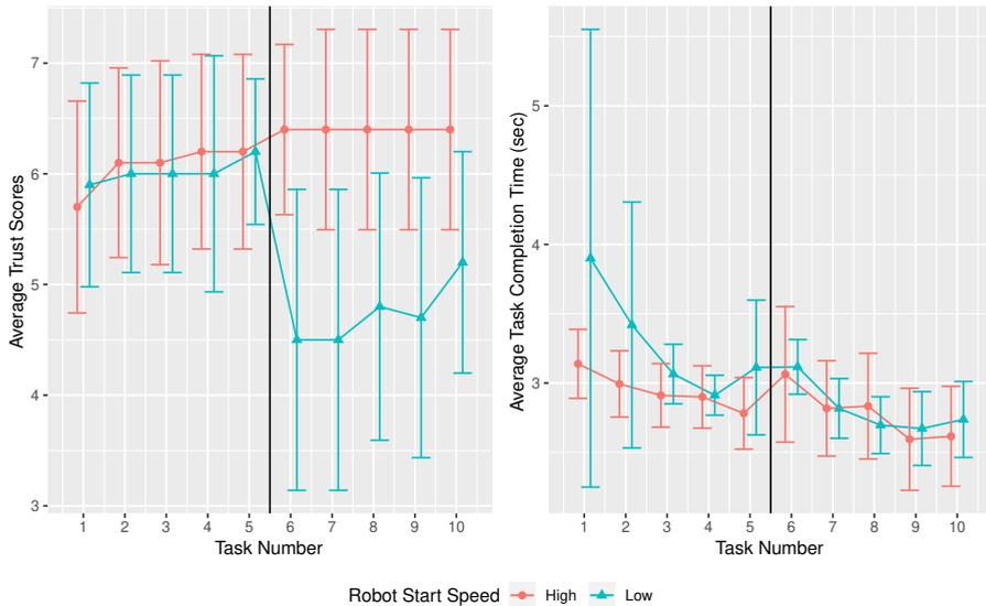
**Fig. G.5:** Left: The average trust rating after each task. Right: The average task completion time in second for each task. Both include error bars and a vertical line marking the mid-point when the robot movement speed changes.
