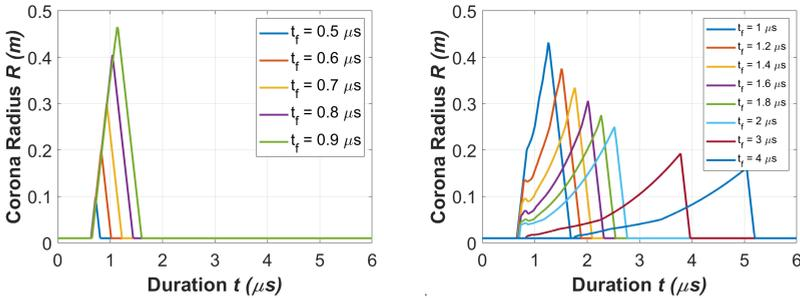
(b) Front time from  $0.5 \mu\text{s}$  to  $0.9 \mu\text{s}$  at an increment of  $0.1 \mu\text{s}$  (c) Front time from  $1 \mu\text{s}$  to  $2 \mu\text{s}$  at an increment of  $0.2 \mu\text{s}$  and to  $4 \mu\text{s}$
