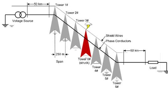
Fig. 2 The demonstration of OHL lines model
