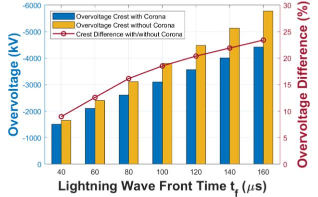
Fig. 9 Overvoltage crests of surge impedance models with and without corona under lightning current of different peaks and the difference of overvoltage crests between the two models
