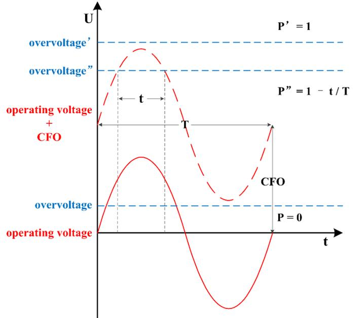
Fig. 6 The demonstration of calculating the backflashover probability under a certain overvoltage
