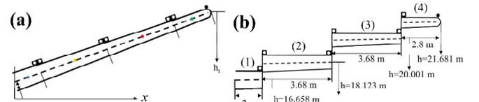
Fig. 3 The sketch of the actual composite cross-arm and the equivalent calculation model.
