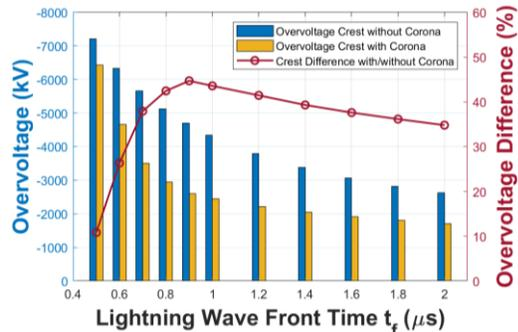
Fig. 7 Overvoltage crests of surge impedance models with and without corona under lightning current of different models and their differences in overvoltage crests between the two models
