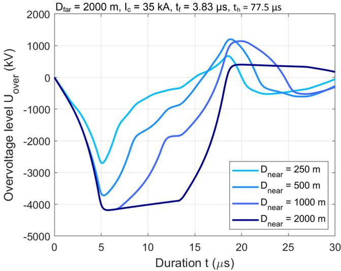
Fig. 5.7: Overvoltage wave fronts of same  $D_{far}$  and different  $D_{near}$ . Source: J1 [120]
