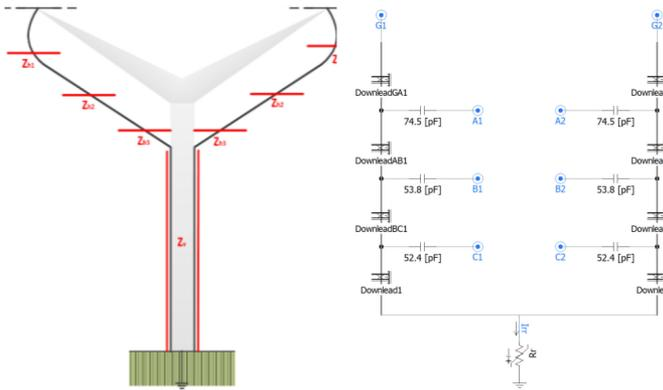
Fig. 3. The demonstration and model of grounding down-leads.
