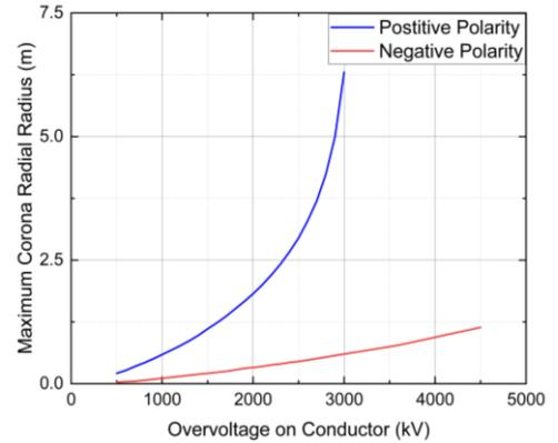
Fig. 2 Maximum corona radius limited by critical streamer-tip electric field under different polarities and amplitude of overvoltage on the conductor
