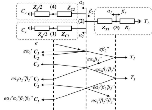
Fig. 8 The lattice diagram for the wave travel of the Y-shaped pylon. (1) and (4) indicate the top of the pylon, (2) is the connection point of the cross-arm and pylon body, and (3) is the bottom of the pylon.  $C_1$  and  $C_2$  are the cross-arms,  $T_1$  is the pylon body.
