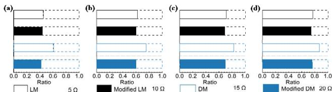
Fig. 10 The ratio  $p$  of  $V_g$  to  $V_{TT}$  calculated by four methods as the tower-footing impedance increases when  $T_f$  is 8  $\mu$ s.
