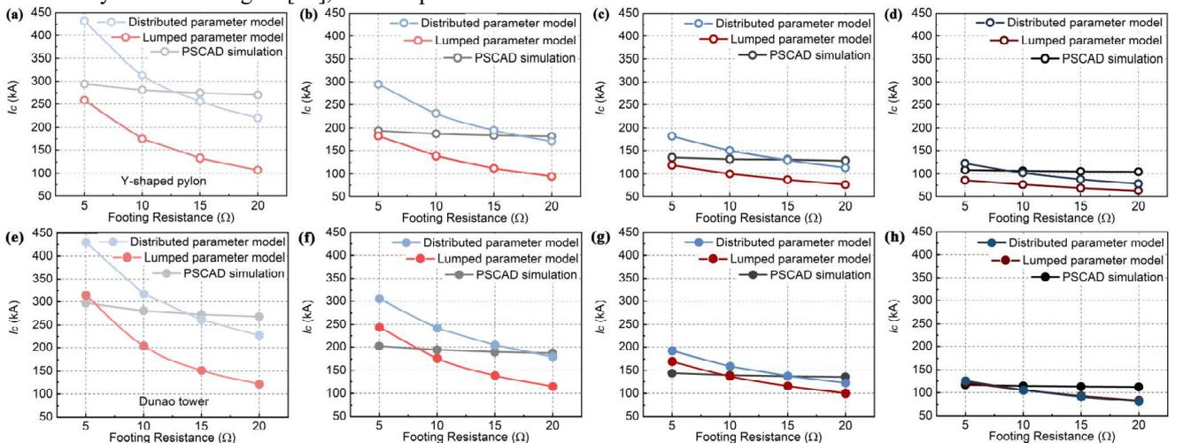
Fig. 6 The comparison of  $I_c$  for Y-shaped pylon obtained by PSCAD simulation, LM and DM with  $T_f$  of (a) 1.2  $\mu$ s, (b) 2  $\mu$ s, (c) 4  $\mu$ s, (d) 8  $\mu$ s.  $I_c$  for Donau tower obtained by simulation and calculation with  $T_f$  of (e) 1.2  $\mu$ s, (f) 2  $\mu$ s, (g) 4  $\mu$ s, (h) 8  $\mu$ s.
