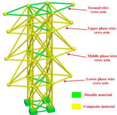
Fig. 1.4: Sketch of a composite-metal hybrid lattice tower [18]
