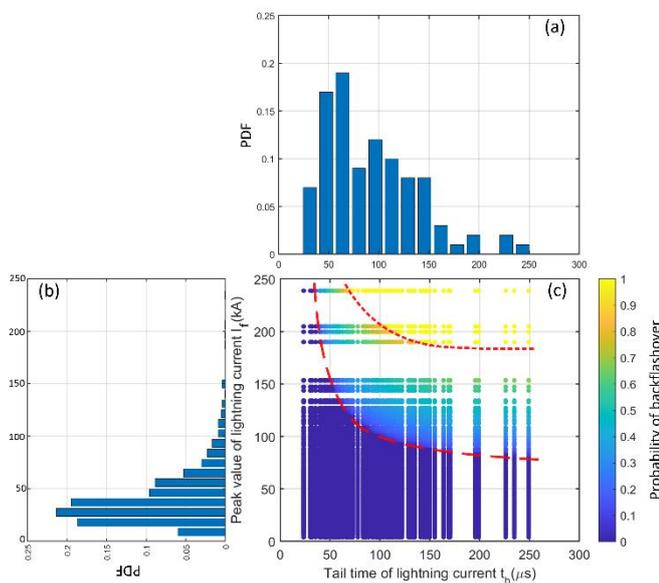
Fig. 8 (a) PDF of tail time of lightning current  $t_h$  (b) PDF of peak value of lightning current  $I_f$  (c) The probability of backflashover under the lightning flashes with different peak values and tail times
