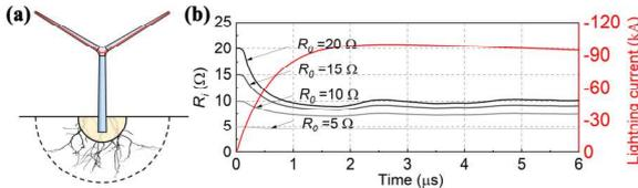
Fig. 4 (a) The schematic of the soil ionization. (b) The  $R_i$  changes with different  $R_0$  when the lightning current passes through the pylon footing electrode (black line), and the lightning waveform (red line).
