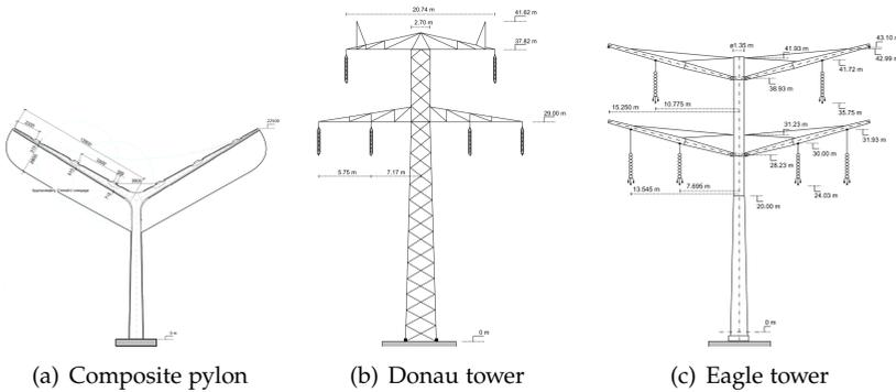
Fig. 5.1: The configuration and dimensions of composite pylon and two steel lattice towers (not in real relative scale). Source: J2 [117]
