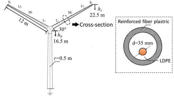
Fig. 2 The parameters of the Y-shaped pylon.
