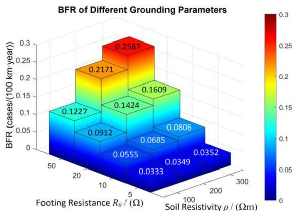
Fig. 4. BFR of OHLs with every pylon grounded of different grounding parameters.
