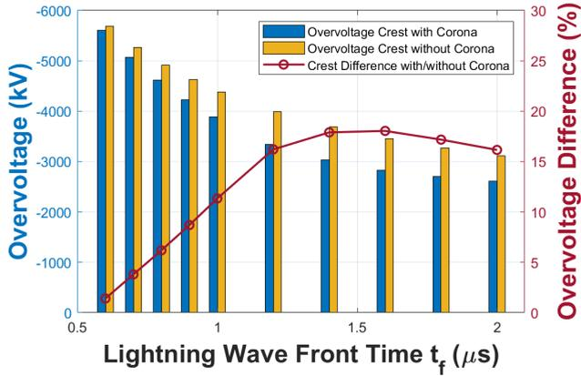
**Fig. 4.8:** Overvoltage crests of surge impedance models with and without corona under lightning current of different front times and the differences of overvoltage crests between the two models. Source: J3
