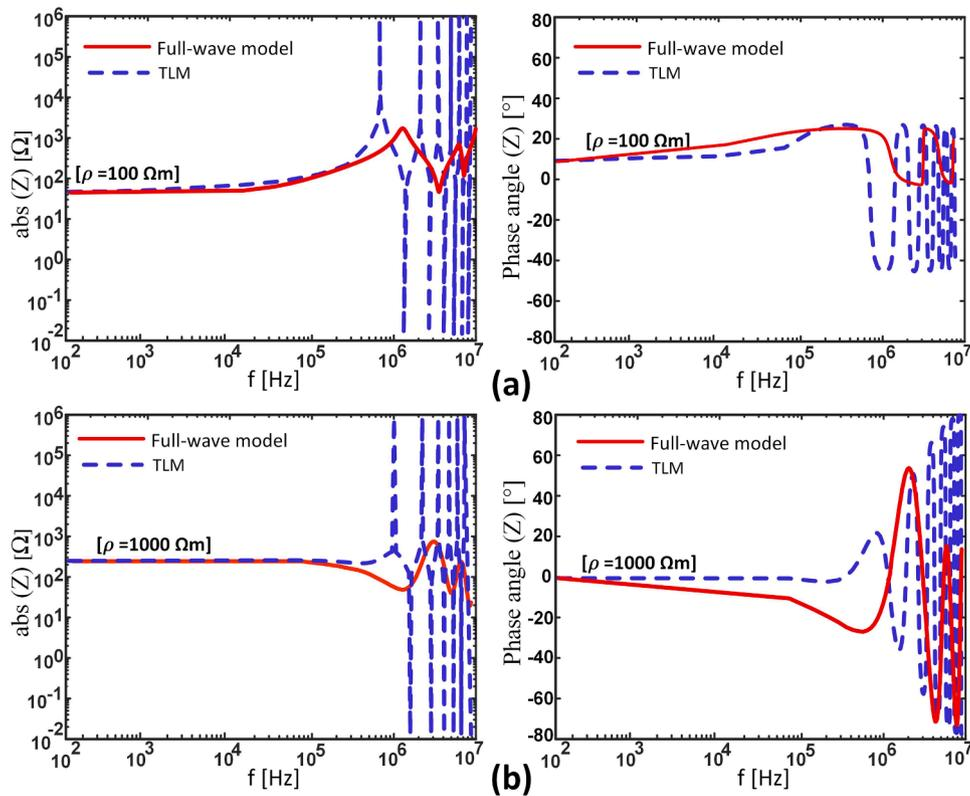
Fig. 8. Harmonic impedance of tower and its connected VGE [absolute value (left column) and phase angel (right column)] shown in Fig. 5(b) [ $\rho= 100 \Omega\text{m}$ ] and Fig. 5(c) [ $\rho= 1000 \Omega\text{m}$ ]. Full-wave model: red line, TLM model: blue dashed line. (For interpretation of the references to colour in this figure legend, the reader is referred to the web version of this article.)
