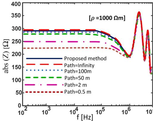
Fig. 6. Integration path effect on the harmonic impedance absolute value of integrated model shown in Fig. 5(c) [ρ= 1000 Ωm].
