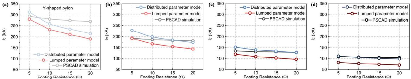
Fig. 9 The comparison of  $I_c$  for Y-shaped pylon obtained by PSCAD simulation, LM and DM with  $T_f$  of (a) 1.2  $\mu$ s, (b) 2  $\mu$ s, (c) 4  $\mu$ s, (d) 8  $\mu$ s considering the effect of soil ionization.
