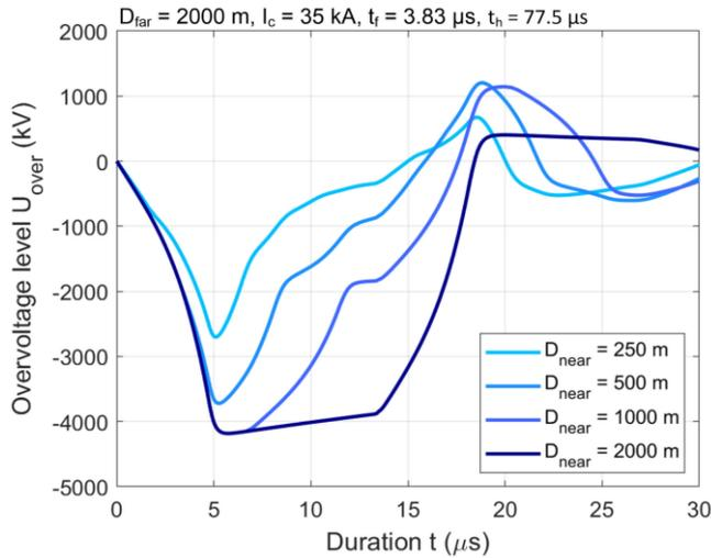
Fig. 7. Overvoltage wave fronts of same  $D_{far}$  and different  $D_{near}$ .
