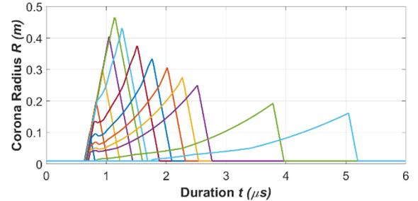
Fig. 5 (a) Corona radius developing processes under different lightning current front times from 0.5 μs to 4 μs
