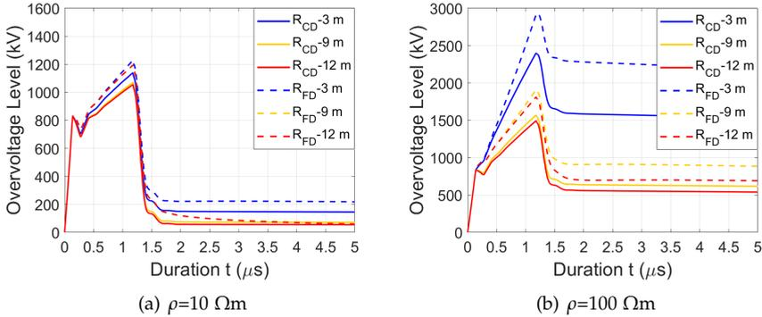
Fig. 3.2: The overvoltage provided CDI model and FDI model with different electrode length
