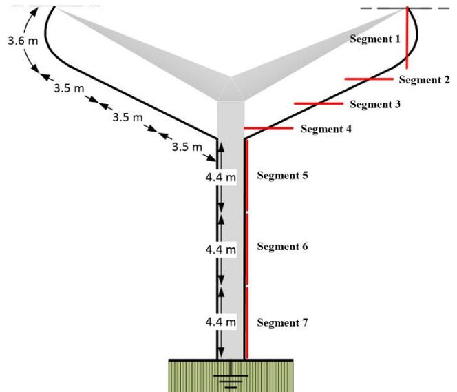
Fig. 2 The demonstration of down-lead segments and dimension
