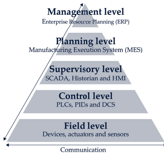
Fig. 1.3: The automation pyramid for a classical manufacturing company. Adopted from Rahman et al. [26].
