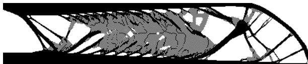
Fig. 2.8: An MBB-beam optimized for compliance suffering from the so-called checkerboards.
