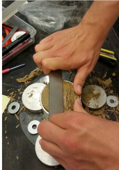
Figure 7.3 Hand trimming of sample.
