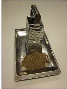
Figure 5.2 Grating the clay to maximise the surface. Figure 5.3 Pugging the clay through a 0.42 sieve.
