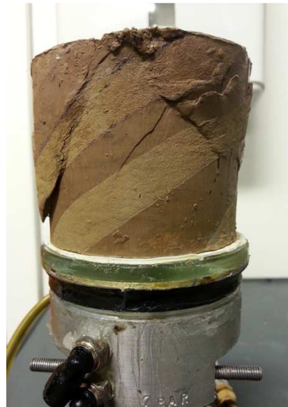
Figure 7.7 Test 5 after shearing.
