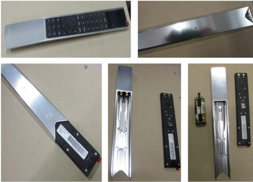
Picture 11-14: The remote control and its disassembly.
