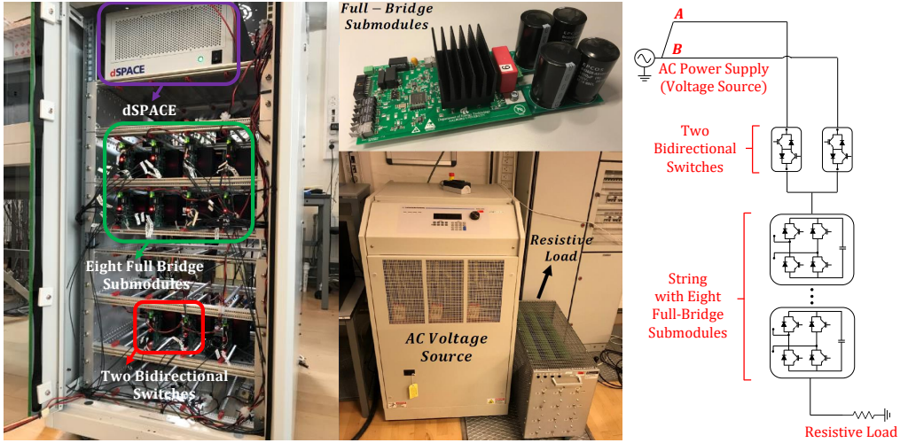
Fig. 29: The left-hand-side image shows a picture of the MMSC test setup, and the right-hand-side image shows a diagram with the main components of the test setup.
