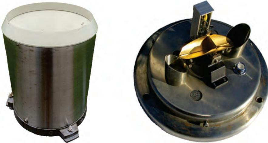
*Figure 3: A Rimco 7499020 tipping bucket rain gauge shown in closed and open state. The last three digits of the model name defines the tipping bucket size, corresponding to 0.2 mm precipitation pr. tip.*
