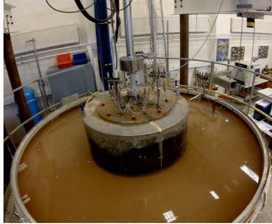
Fig. C.1: Laboratory installation test of a bucket model
