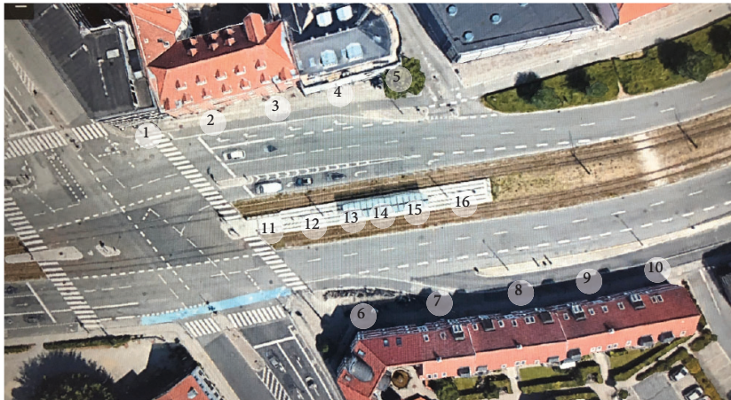
Figure 20. Plan, illuminance measurements on pavement along facades and platform floor (Google Maps)
