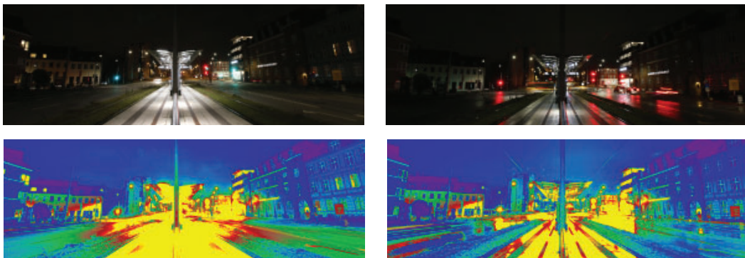
Figure 24. Photos and luminance maps, view from rear end of Nørreport station. Left, existing lighting setting. Right, dimmed lighting setting.
