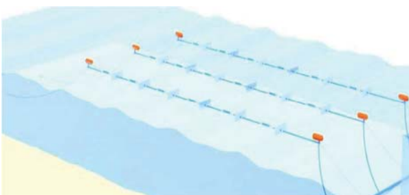
Fig. 2 - WavePiston future installation as a wave-farm. Note that for illustration purposes only 6 plates (modules) are drawn to each string. In a real WavePiston installation up to 50 collectors may be attached to each string in order to get a full benefit.
