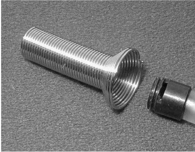
FIG. 1. The thermo-expandable Ni–Ti stent is shown together with insertion kit to mount over the flexible cystoscope. Initially the stent is a straight cylinder. The stent shown here has been flushed using water at 60 °C. This causes the collar to expand at the lower end of the stent. The expanded collar locks the stent position in the prostate.
