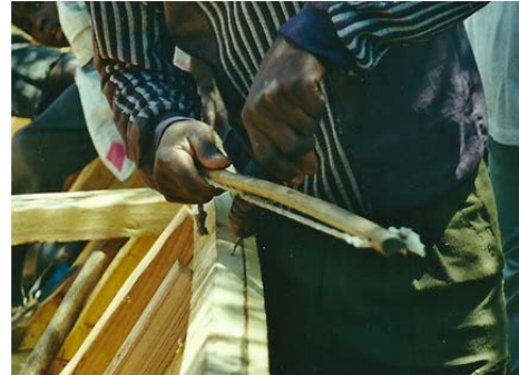
Hand operated, locally made drilling tool
