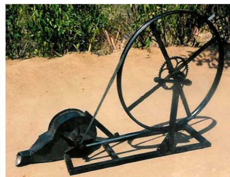
Proto-type bicycle wheel operated fan
