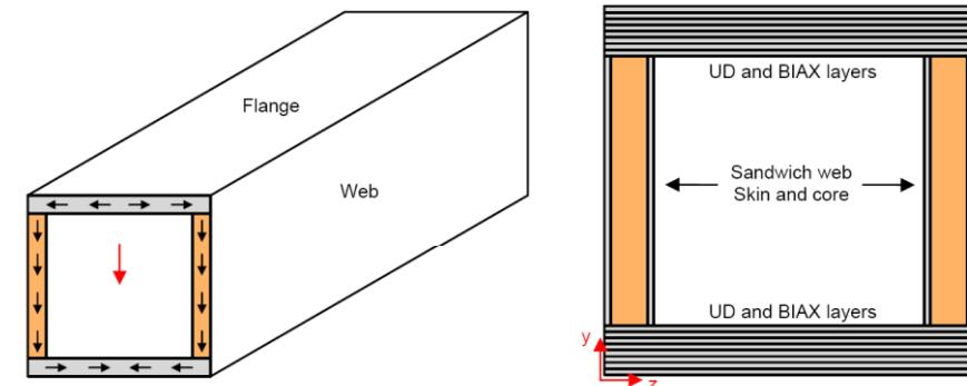
Figure 6-3: The directions of the shear stresses in the composite cross section plane.
