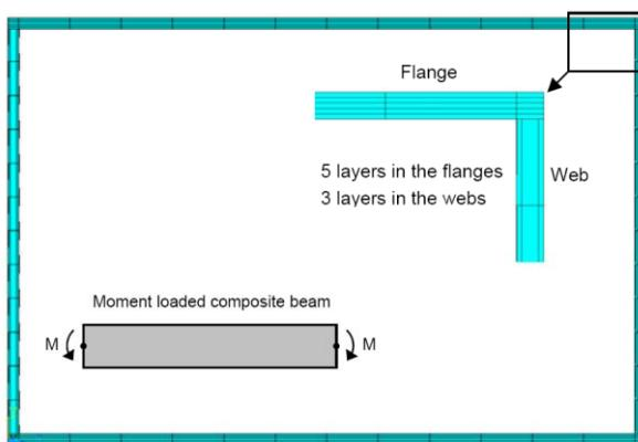
Figure 5-5: Cross section of the FE model with layered elements. ANSYS plot.
