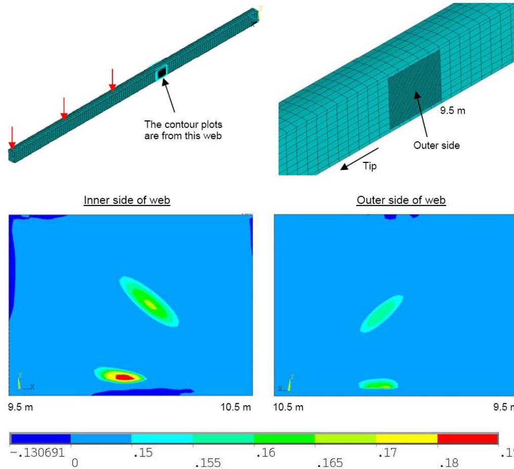
**Figure 9-8:** Contour plots from ANSYS of the separation of the cohesive elements. Skin-debonding is seen in the middle of the web and in the web towards the compression flange.
