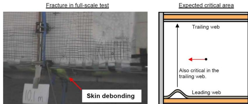
Figure 9-1: Fracture in the leading web towards the compression flange. Skin debonding failure.
