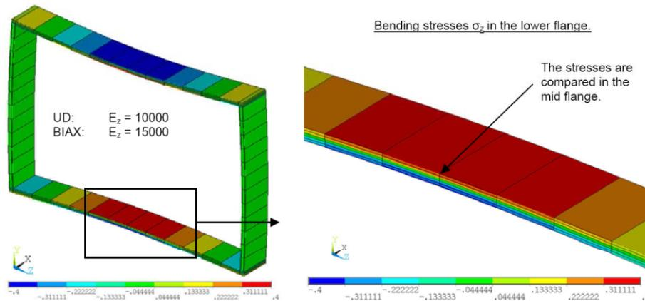
Figure 5-9: Contour plot from ANSYS of the normal stresses  $\sigma_z$  in the lower flange. The layer on the outer side has number 1 and the layer on the inner side has number five.
