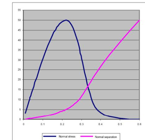
Figure 7-5: Left: Deformed figures from ANSYS with growth of delamination in mode I loading. The separation is scaled with a factor 10. Right: The normal stress and separation as function of the sub step. The normal separation is scaled with a factor 100.
