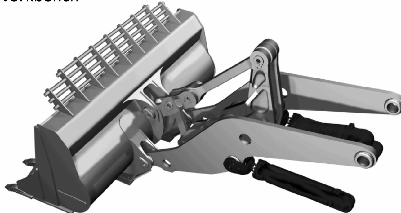
Figure 2: Load unit of a Volvo Wheel Loader with 16 journal bearings.
