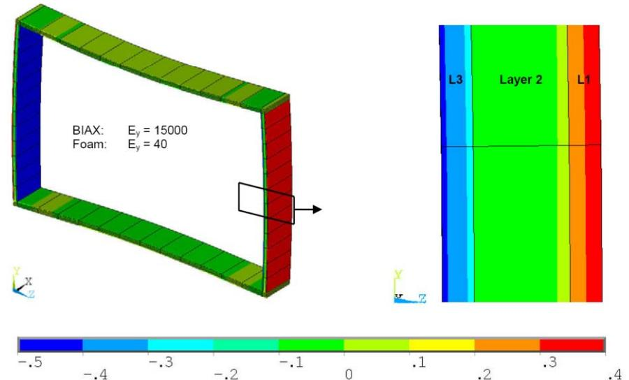
Figure 5-10: Contour plot from ANSYS of the normal stresses  $\sigma_y$  in the mid web.
