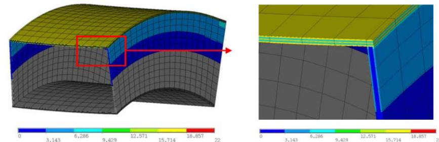
Figure 5-7: Contour plot from ANSYS of the longitudinal stresses  $\sigma_x$  in the composite beam. The grey area on the beam indicates the boundary between the tensile and compression stresses.
