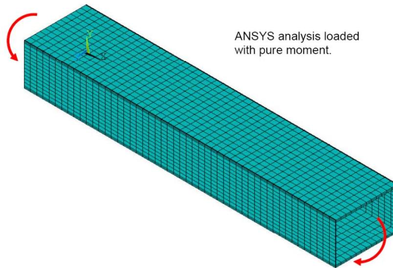
**Figure 4-25:** The ANSYS analysis used for comparisons. A rectangular hollow beam loaded with pure moment.
