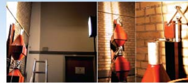
Hot-sphere anemometers placed in the jet-wind tunnel.
