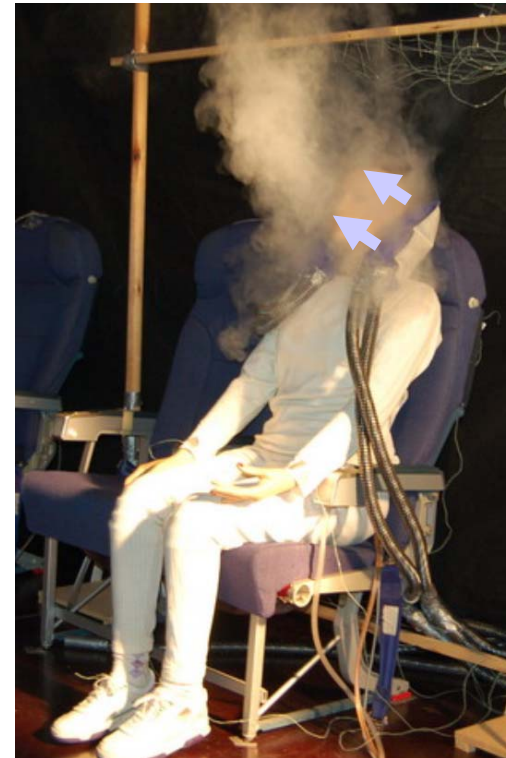
Low velocity supply to the boundary layer
