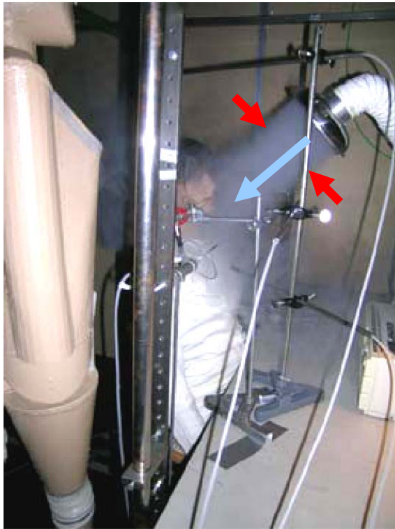
High momentum flow with entrainment
