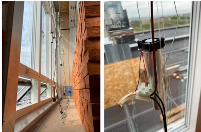
Fig. 6. Air temperature measurement in the integrated solution (a) DSF cavity (b) DCV plenum (c) Thermocouples type K with shielding tubes.
