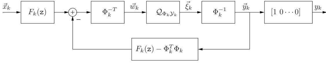
Fig. 2. MH quantization implemented using a noise-shaping architecture.
