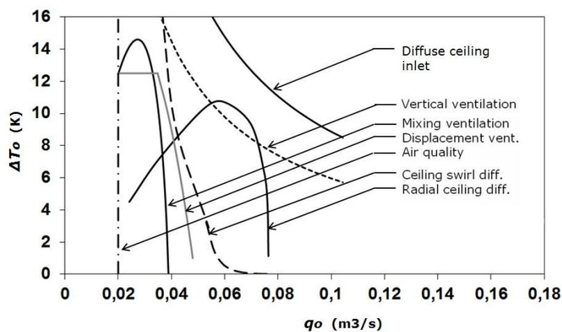
Figure 12. Design chart for the six different air distribution systems. Air quality requires that  $q_o$  is larger than  $0.02 \text{ m}^3/\text{s}$ .
