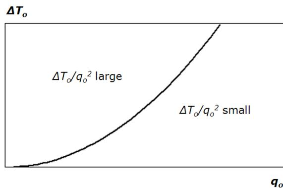
Figure 2. Determination of airflow in a room with a given  $a_o/A$  ratio based on the critical Archimedes number. Stratified flow or large mixing effect can take place in the left side of the graph while large mixing effect can take place at the right side of the graph due to high supply momentum.
